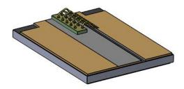
SkyEra delivers chip on submount diode lasers, employing AuSn bonding and P Down package with multiple advantages of high reliability, stable output power, high power, high efficiency, long lifetime and high compatibility, and are widely applied in the market.
