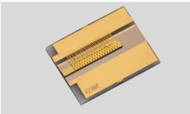
SkyEra delivers TY-915 $\pm$ 10nm-22.0W-25C-COS-01 chip on submount diode lasers, employing AuSn bonding and P Down package with multiple advantages of high reliability, stable output power, high power, high efficiency, long lifetime and high compatibility, and are widely applied in the market.
