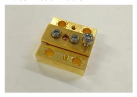
SkyEra delivers TY-825NM+/-05NM-60.0W-25C-CS single bar diode lasers, employing AuSn bonding technology with multiple advantages of low smile, stable output power, high power, high efficiency, long lifetime and high compatibility, and are widely applied in the market.
