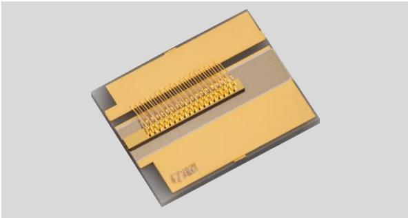
SkyEra delivers TY -808±3nm-5.0W-25C-COS-200 chip on submount diode lasers, employing AuSn bonding and P Down package with multiple advantages of high reliability, stable output power, high power, high efficiency, long lifetime and high compatibility, and are widely applied in the market.
