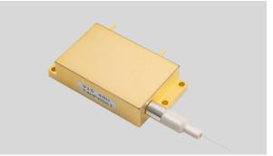
SkyEra delivers TY-0450+/-10NM-20.0W-25C-105-0.22NA diode lasers employing professional coupling technology, that enjoy multiple advantages, e.g., compact design, stable output power, high power, high efficiency and convenient packaging. These laser diode modules can provide solutions for fiber laser applications and direct suppliers.
