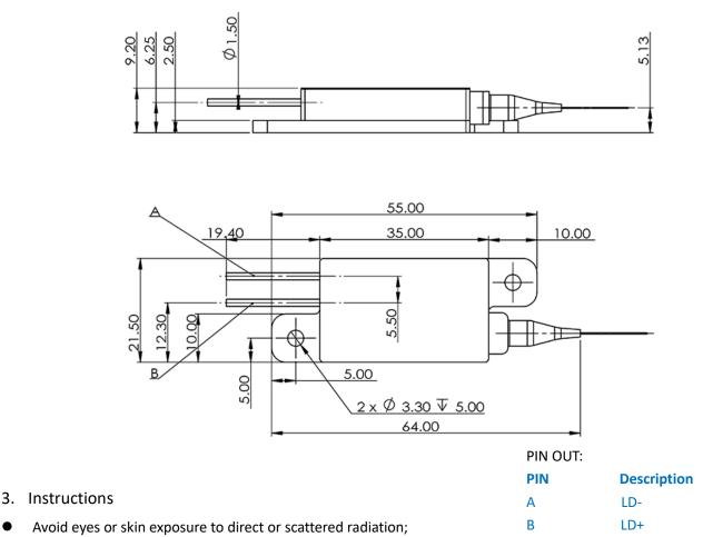
• ESD protection is required for transportation, storage and operation; short-circuit protection between pins is required
