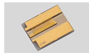
SkyEra delivers TY-975  $\pm$  05nm-12.0W-25C-COS-DG-01 chip on submount diode lasers, employing AuSn bonding and P Down package with multiple advantages of high reliability, stable output power, high power, high efficiency, long lifetime and high compatibility, and are widely applied in the market.
