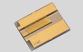
SkyEra delivers chip on submount diode lasers, employing AuSn bonding and P Down package with multiple advantages of high reliability, stable output power, high power, high efficiency, long lifetime and high compatibility, and are widely applied in the market.
