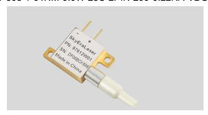
SkyEra delivers TY-808+/-01NM-9.0W-25C-2PIN-200-0.22NA-VBG diode lasers employing professional coupling technology, that enjoy multiple advantages, e.g., compact design, stable output power, high power, high efficiency and convenient packaging. These laser diode modules can provide solutions for fiber laser applications and direct suppliers.
