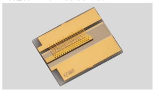
SkyEra delivers TY -785 $\pm$ 05nm-2.0W-25C-COS-100 chip on submount diode lasers, employing AuSn bonding and P Down package with multiple advantages of high reliability, stable output power, high power, high efficiency, long lifetime and high compatibility, and are widely applied in the market.
